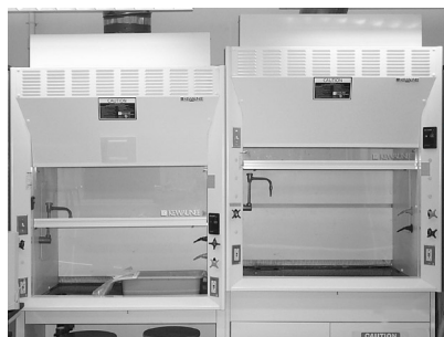
Low-rise exhaust hood (L) permits easier access for wheelchair and other handicapped students.
