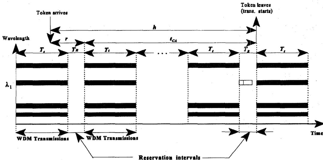
Figure 2: Interlaced WDM transmissions and reservation intervals.
