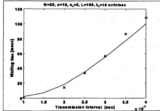
Figure 8: Mean waiting time ( $W_Q$ ) vs transmission interval ( $T$ ).
