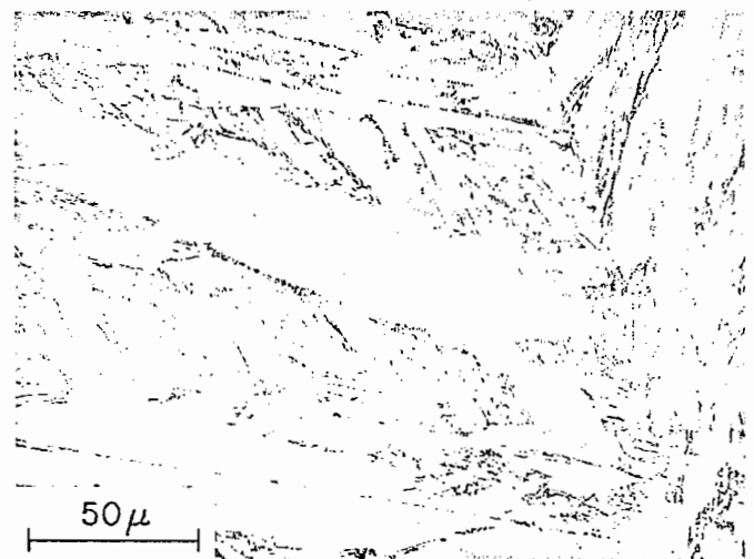
Fig. 1—Midribbed martensite in Fe-25 Ni-8 Cu alloy.
