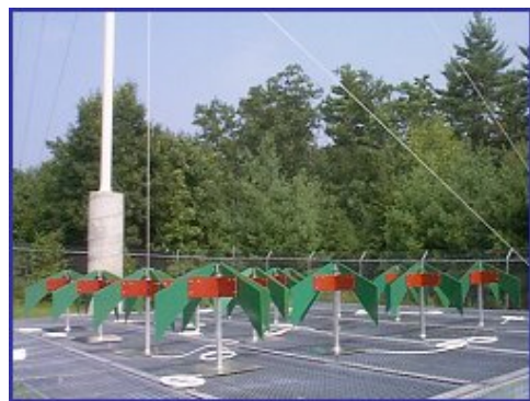
Prototype array of low-frequency dipoles designed to operate at 80–300 MHz.
