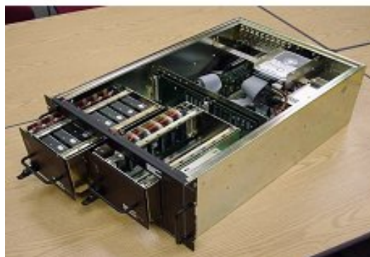
Haystack's Mark 5 data system used for disk-based recording and e-VLBI.
