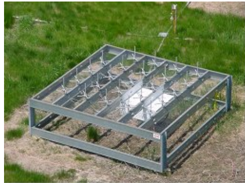
One station of the Deuterium array showing the 24 dipoles and digital receiver box.
