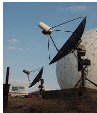
Radio interferometry using two small radio telescopes.
