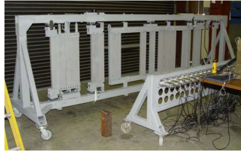
Large coded aperture for fissile material detection.
