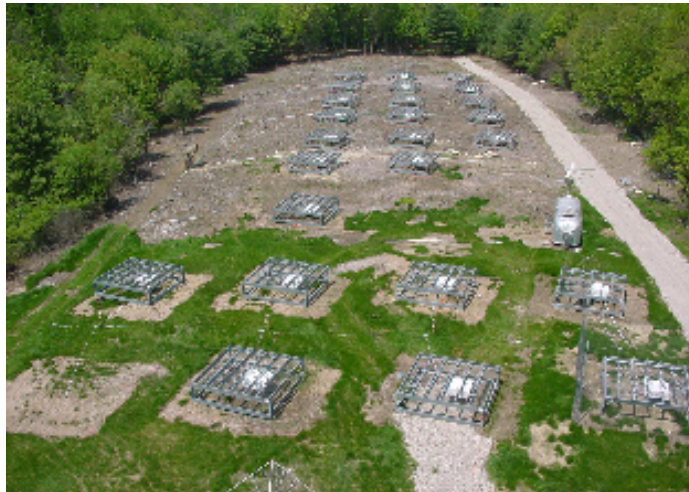
Figure 1. Deuterium array at Haystack showing the 24 stations each with 24 dual-polarized dipoles, coupled to digital receivers at 327.4 MHz. The trailer contains the RFI detection system, which consists of 12 Yagi antennas pointed every 30 degrees.
