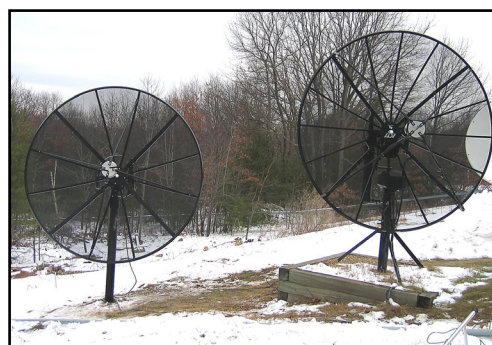
Figure 8. A two-element radio interferometer for educational projects using Haystack's small radio telescopes.
