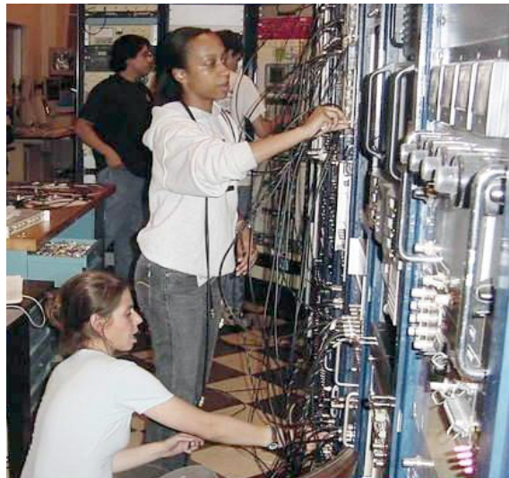
Figure 5. MIT students setting up radar electronics for experiments at the Arecibo Observatory in Puerto Rico.
