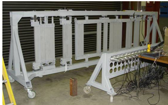
Coded aperture for fissile material detection.
