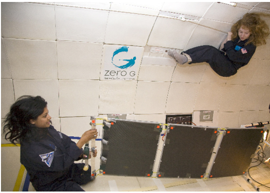
Figure 4. Aboard the Zero-G aircraft, conducted in conjunction with AeroAstro's Giant Leaps Apollo anniversary events, Tina Srivastava (left) and Jillian James test microgravity deployment of a solar panel for an undergrad satellite project. (Steve Boxal/Zero Gravity Corp. photo)
