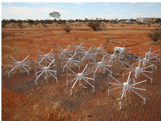
Figure 1. An antenna tile of the MWA with the electronics hut and office trailer visible in the background, at the MWA site in Western Australia. The system is currently powered by a 35 kVA diesel generator provided by Australian partners. Each tile consists of 16 individual dual-polarization dipoles and an electronic beam forming unit that can steer the tile beam in any direction across the sky (the box on the far side of the tile in this photo). The full MWA will comprise 512 such tiles.
