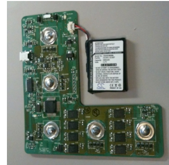
Figure 10. A photo of the wearable, wireless cardiac monitor. The monitor is coated in Parylene C to protect it from water and sweat that may come in contact with the circuits.
