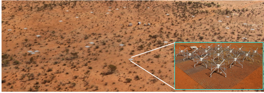
Figure 1. Aerial view of the MWA 32-tile system located on the radio-quiet Murchison Radio Observatory site in Western Australia. The prototype 32-tile system is laid out in a rough circle 300 meters in diameter, and the full system to be completed in 2011 will comprise 512 tiles spread over an area 3 kilometers in diameter. Each tile (inset) consists of 16 individual dual-polarization dipoles and an electronic beam forming unit that can steer the tile beam in any direction across the sky.
