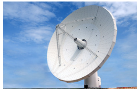
Figure 6. Photo of the cryogenic “Eleven” feed being considered for the 12-meter geodetic antenna system.
