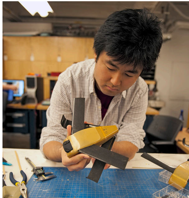
Master's candidate Tony Tao folds the wings of a Locust, a micro UAV developed by AeroAstro students working with Lincoln Laboratory and Aurora Flight Sciences. The vehicle was fabricated using equipment in AeroAstro's Gelb Lab.
