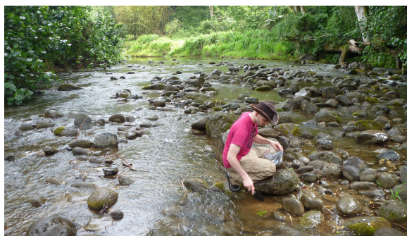
Postdoctoral researcher Ken Ferrier collects a sample of sediment from a river on the Hawaiian island of Kaua'i. Laboratory measurements of the isotope ^3\text{He} in grains of olivine (also known as the gemstone peridot) are used to measure the erosion rate of the river basin over the past several thousand years as part of a comparison of erosion on the dry and wet sides of Kaua'i, which has one of the steepest rainfall gradients in the world.
