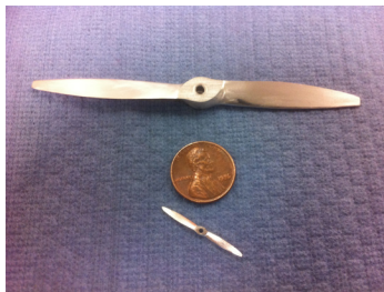
Figure 4. Two aluminum propellers made in the Central Machine Shop.
