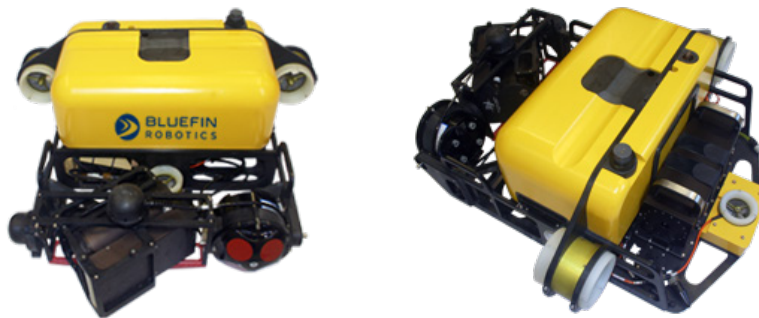
Figure 1: Small, hovering AUVs designed for inspecting ship hulls for explosives or contraband.
