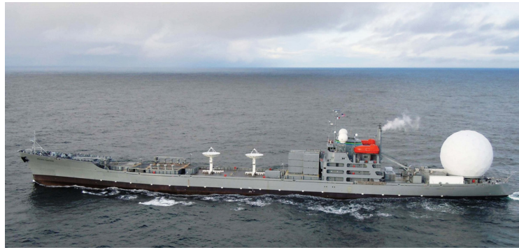
Figures 4a, 4b. The XTR-1 radar installed on the stern of the Pacific Tracker.
