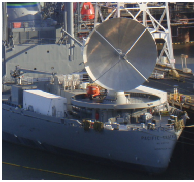
Figures 4a, 4b. The XTR-1 radar installed on the stern of the Pacific Tracker.
