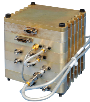
Figure 10. Researchers in the Tactical Systems mission area are developing a prototype Ku-band radar.
