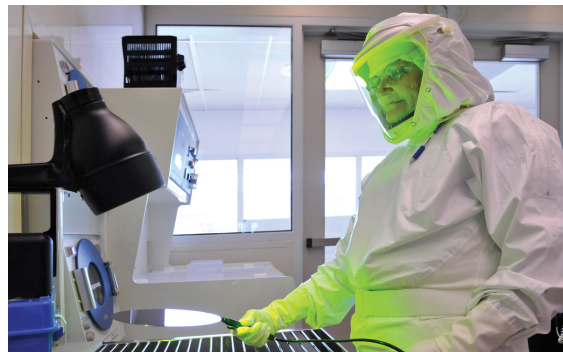
Figure 8. In the re-outfitted Microelectronics Laboratory, a technician performs bright-light inspection of a 200 mm wafer prior to 3D bonding.
