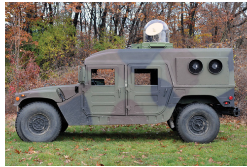
Figures 5a, 5b. A researcher operates the Portable Army Communications-on-the-move Terminal Block 1 mobile SATCOM terminal (atop vehicle), demonstrating the ability to have mobile communications that are robust to disruption by jamming or other attacks.
