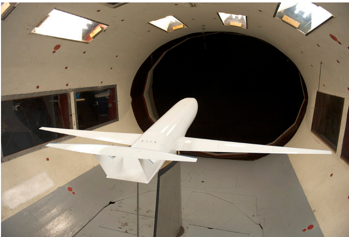
A 1:10 model of the D-8 commercial aircraft concept is prepared for testing in AeroAstro's Wright Brothers Wind Tunnel. Designed by an MIT-led team, the 737-size plane could burn 70 percent less fuel than current aircraft while reducing noise and nitrous oxide emissions.
