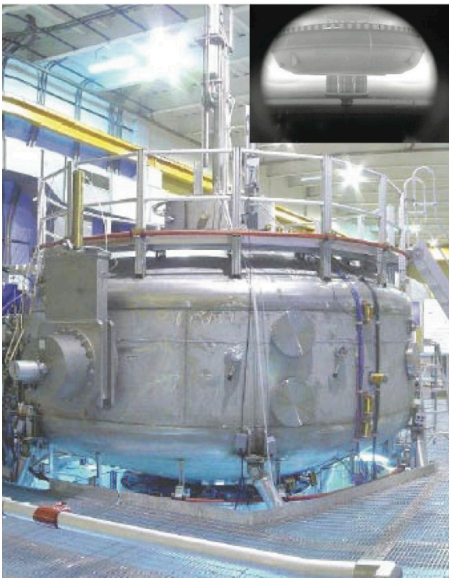
Figure 2. A "laboratory magnetosphere" using a half-ton levitated superconducting ring.
