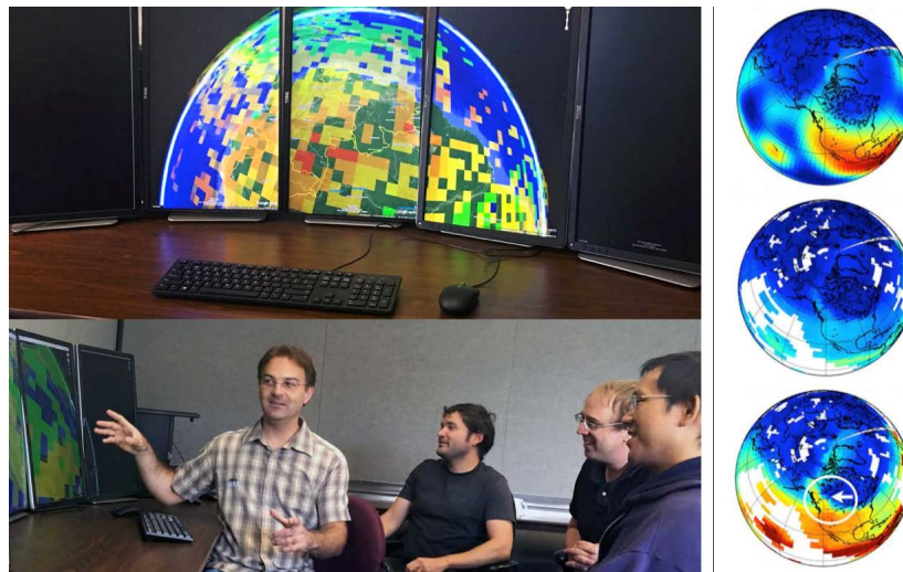
Victor Pankratius (left) and his group visualizing current conditions of the Earth's ionosphere in 3D. At right is an illustration of the same total electron content data set and how choice of workflow algorithms and parameters can affect the visibility and discovery of interesting geophysical phenomena. This is where humans can count on more efficient algorithmic support using MIT Haystack's computer-aided discovery system.
