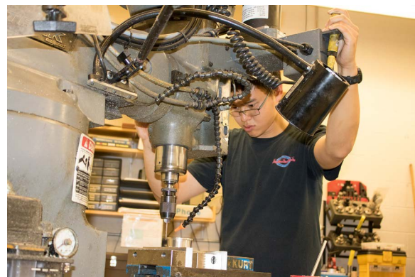
Mitchell Hsing (G), a member of the Schmidt Research Group, mills an aluminum component at the Edgerton Student Shop. The Schmidt Research Group is designing and fabricating micro-vacuum pumps that can be used for portable diagnostic instruments that require vacuum processing of samples.
