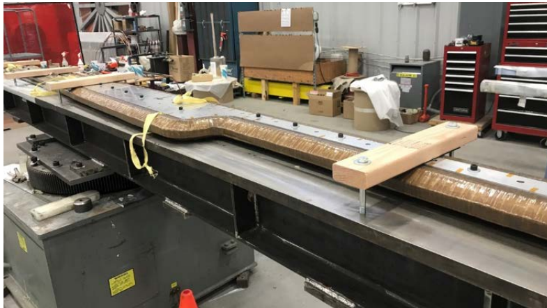
The prototype coil for the MOLLER experiment hybrid toroid on its winding frame, mounted on a steel support beam for shipping. From Scott Morley.
