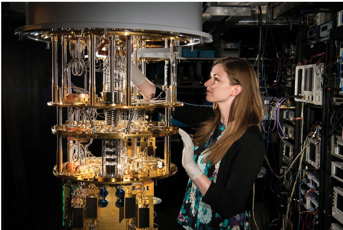
Figure 8. Bethany Huffman adjusts the dilution refrigerator that cools qubit circuits to twenty thousandths of a degree above absolute zero when operating. Lincoln Laboratory's 3D approach to fabricating qubits is enabling more flexible and complex circuitry needed to advance superconducting quantum computers.
