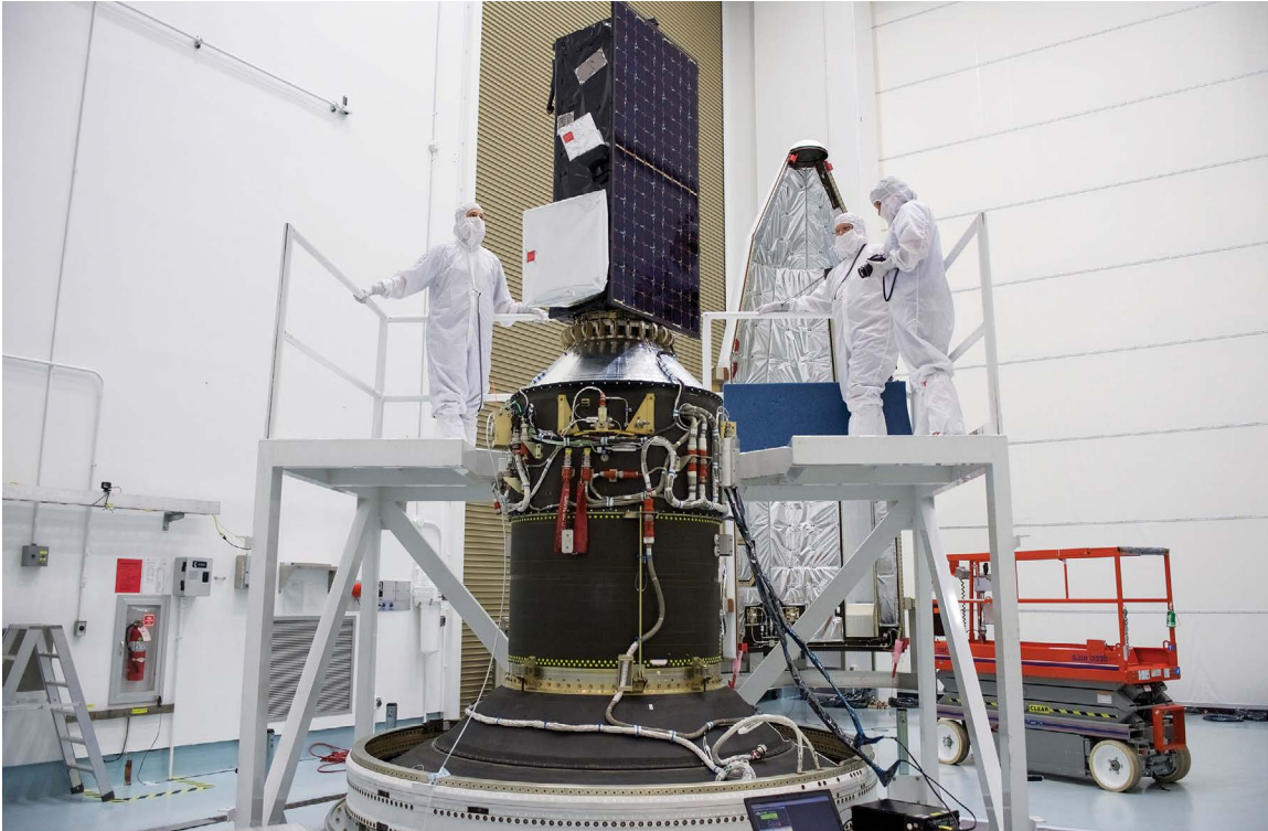
Figure 11. Lincoln Laboratory staff performed the final closeout and inspection of the SensorSat space vehicle during integration on the Minotaur rocket from which it was launched at Cape Canaveral, FL. SensorSat is now providing data for space situational awareness.
