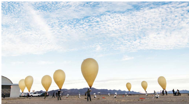
Figure 4. The HALO (High-altitude Attritable Link Offset) program successfully demonstrated the first balloon-based communications relay array. Ten low-cost balloon payloads used distributed adaptive array processing techniques to achieve over-the-horizon communications despite co-channel interference.
