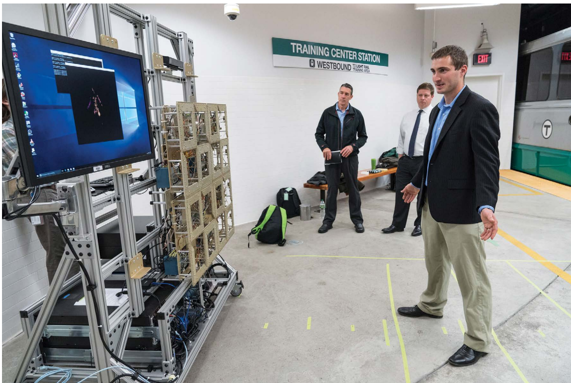
Figure 9. Engineers test a microwave imaging system in a Massachusetts Bay Transportation Authority training center. The system collects radar reflections off liquid, metal, or plastic objects concealed on pedestrians; algorithms process the imagery in real time to determine whether the objects are threat items.
