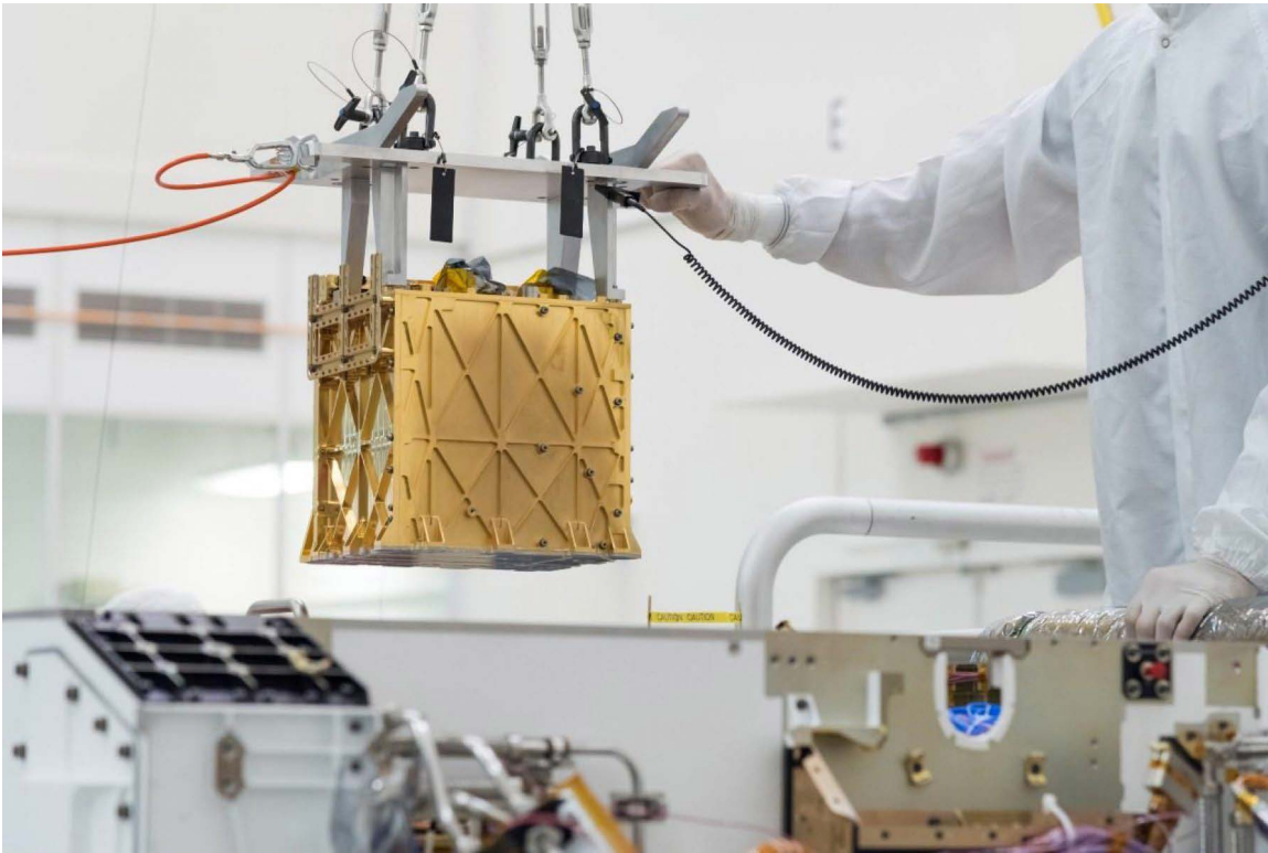
Figure 11. MOXIE, the Mars Oxygen In-Situ Resource Utilization Experiment.
