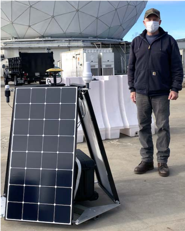
Figure 9. Haystack scientists and engineers designed an autonomous geodetic-quality Global Navigation Satellite Systems (GNSS) buoy, and built and shipped twelve of the Sea Ice Dynamic Experiment (SIDEx) buoys in March 2021 to remote northern Alaska to learn more about the physics of sea ice in the Arctic Ocean.
