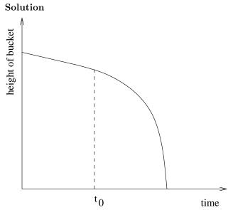
At first, the height of the bucket decreases at a constant rate (linearly) because the bucket is being lowered with a constant speed. After the rope is cut at time  $t_0$ , the bucket experiences a constant downward acceleration, so its height decreases at an increasing rate (quadratically, concave down).
