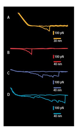
Figure 9: Typical AFM force curves for adhesion proteoglycan (AP) molecules on both the AFM tip and on a mica substrate. The retracting part of the force curves shows discrete jumps as AP-AP bonds are broken. Reprinted by permission, reference (57). Note that the NanoScope MultiMode AFM can resolve picoNewton-scale forces.
