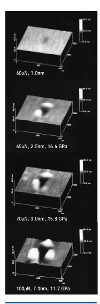
Figure 14: NanoScope AFM images of silicon 111 surfaces after indentation with a diamond AFM tip with loads of 60, 65, 70, and 100μN. The smallest load produced an indentation only 1nm deep, the largest load created an indentation about 7nm deep. Reprinted by permission, reference (89).
