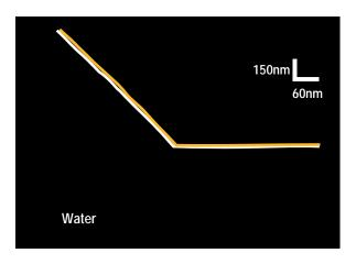
Figure 5: Measurement of the forces between an AFM tip and a mica surface in air and water. The measurement in air shows a large adhesive force due to capillary forces from the liquid contaminant layer on the surface. Once the whole cantilever probe is immersed in water, capillary forces are mostly eliminated and adhesion is substantially diminished. From A.L. Weisenhorn, reference (1).
