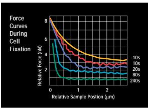
Figure 12: (A) and (B) show the surface of an MDCK monolayer before (A) and after (B) glutaraldehyde fixation. The surface (B) is markedly rougher. The graph shows sequential AFM force measurements on the cell monolayer during fixation. The force curves become increasingly steep over time, illustrating the mechanical stiffening of the monolayer during fixation. This work was done on a NanoScope MultiMode AFM. Reprinted by permission, reference (70).
