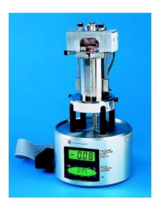
Figure 3: Digital Instruments MultiMode<sup>TM</sup> AFM, optimized for high resolution force measurements and topographic imaging.
