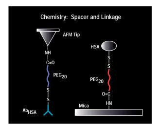
Figure 11: (Top) Schematic of "sensor force microscopy." A biological sensor molecule, in this case  $Ab_{HSA}$ , is attached to an AFM tip with a molecular tether, the  $PEG_{20}$  molecule. The sensor molecule is scanned across the surface while force measurements detect whether a binding event occurs when a target molecule is encountered. (Bottom) Details of chemical link of sensor and target molecules. Reprinted by permission, reference (63, 64).
