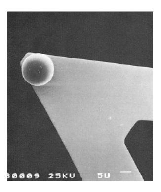
Figure 7: The AFM can measure forces on colloidal particles. In this case, a silica bead was glued to an AFM cantilever to probe the force between the bead and water droplets or air bubbles. Reprinted by permission, reference (44).
