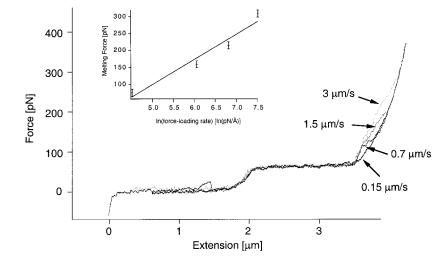
FIGURE 4 Superposition of four extension traces of the same piece of  $\lambda$ -BstE II digest DNA at different pulling velocities: 3, 1.5, 0.7, and 0.15  $\mu$ m/s. The force at which the melting transition occurs depends on the pulling velocity, ranging from 68 pN at 0.15  $\mu$ m/s to ~300 pN at 3  $\mu$ m/s. *Inset*: Melting force versus logarithm of the force loading rate.
