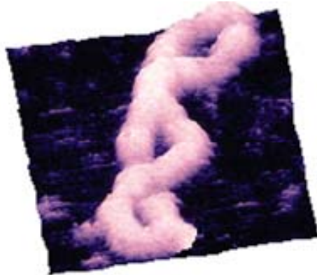
The high resolution of the SPM is able to discern very subtle features such as these two linear dsDNA molecules overlapping each other. 155nm scan. Image courtesy of W. Blaine Stine
