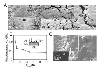
**Fig. 4.** Microindentation of the shell of *C. squamiferum..* (*A*) SEM images of residual indents of Vickers microhardness experiments with load normal to the shell surface (maximum load approximately 9.8 N, depth 62  $\mu$ m). (*B*) Measured Vickers hardness as a function of the maximum applied load (error bars indicate standard deviation). (*C*) SEM images of residual indent (load applied normal to cross section of GL). *Inset* shows the fracture processes in the GL.
