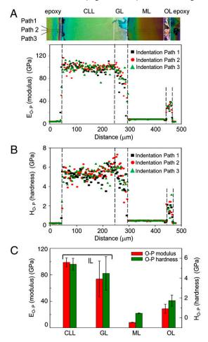
**Fig. 2.** Mechanical properties of the individual layers of the shell of *C. squamiferum..* (*A*) Spatial distributions of O-P modulus and (*B*) hardness through the cross section (top optical microscopy image) for three different spatial pathways. (*C*) Pooled statistics (mean values and standard deviations) of O-P modulus and hardness for each layer.
