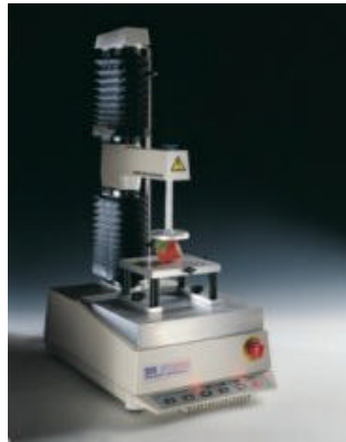
Figure 2.9 Picture of TEE32 Texture Analyzer used during for uniaxial analysis.
