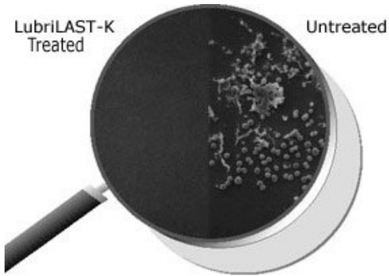
Figure 5.2 SEM Image of bacterial adhesion with and without silver ions present. 31
