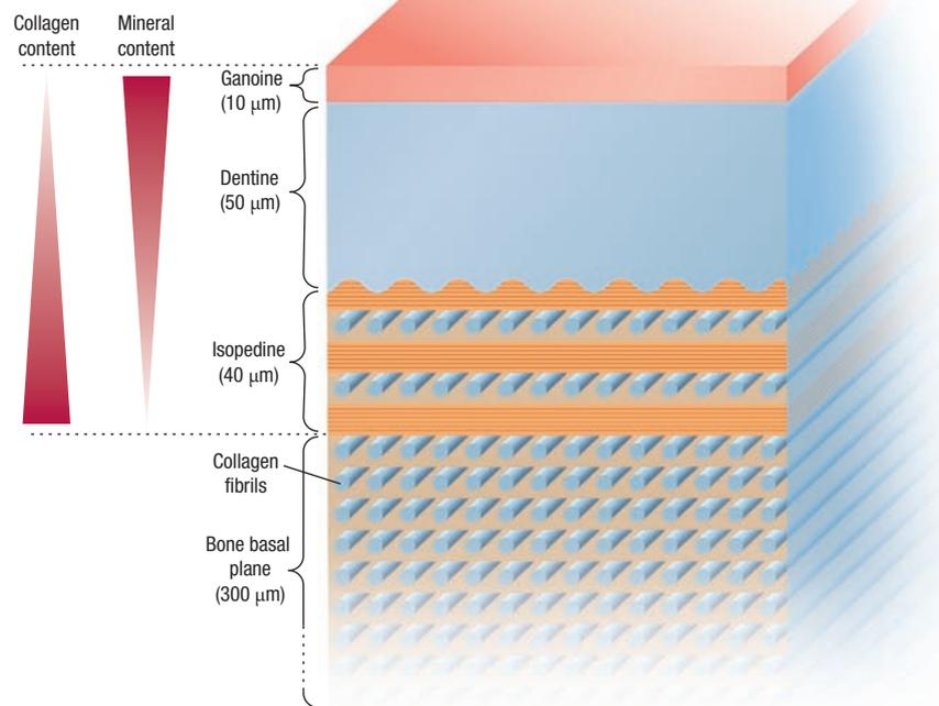
**Figure 2** The four different layers that make up the fish’s scales. The outer layer is composed of ganoine, the next is formed of more compliant dentine that dissipates energy plastically, the third layer is isopedine and the inner layer is formed of bone lamellae. From the outer to the inner surfaces, the mineral content decreases and the collagen content increases, for the first three layers.
