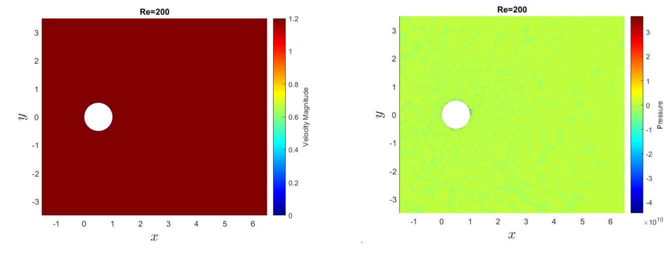
As expected, catastrophic failure of the solver! (does not converge at all, residual explodes)
