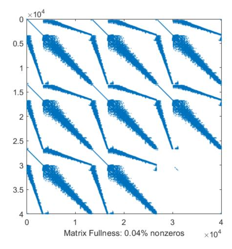
Then, at each iteration k:  $\mathbf{x}^{k+1} = \mathbf{x}^k - \mathbf{J}^{-1}(\mathbf{x}^k)\mathbf{R}(\mathbf{x}^k)$ . Iteration stops when:
