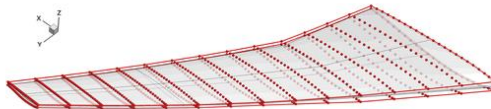
Figure 3. FFD volume and 720 geometric control points
