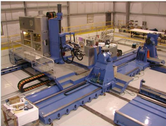
Figure 2. Fiber placement machine.
