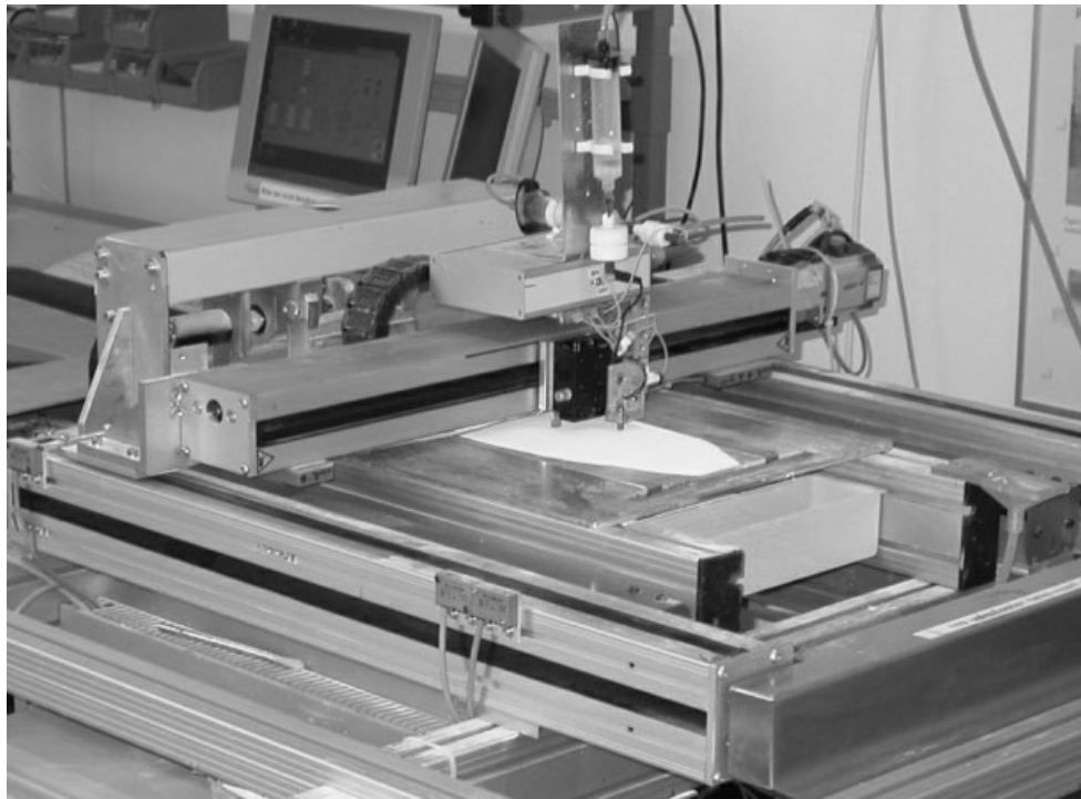
Figure 1. Flexible 3D printing test setup used for process investigation.
