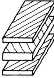
Fig. 5 – A multi-ply laminate composed of individual laminae, each possibly of a different material and oriented in different directions.
