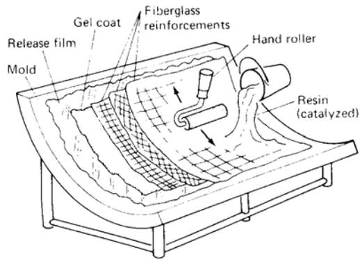
Fig. 2 - Wet hand lay-up process (Lubin, p. 346)
