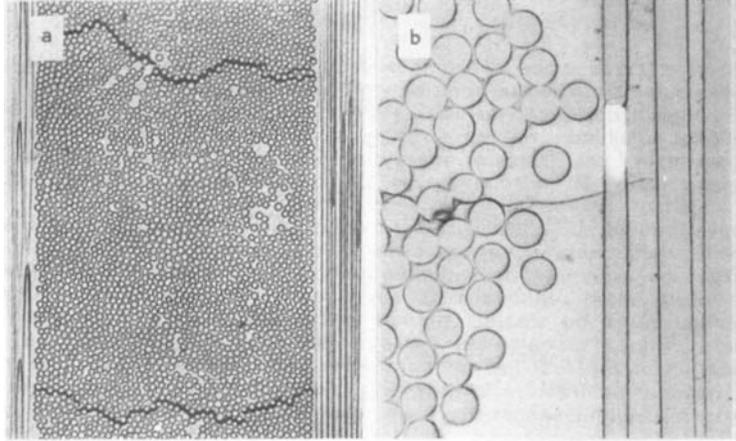
Fig. 1 - A crossplied FRP laminate, showing nonuniform fiber packing and microcracking (from B. Harris, *Engineering Composite Materials*, The Institute of Metals, London, 1986).
