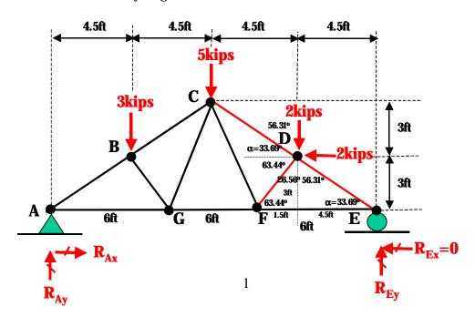
2. Determine support reactions using the equations of static equilibrium
