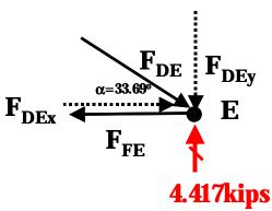
5. Write and solve equations of static equilibrium\* for diagram drawn in step 4.
