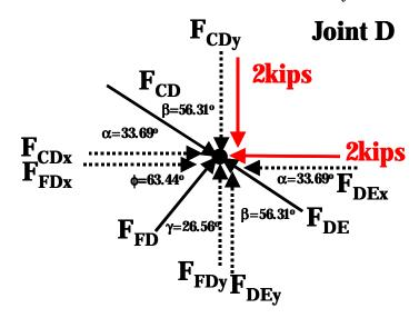
From geometry :  $F_{DEx}=F_{DE}\cos\alpha=0.832F_{DE}=6.625$  kips
