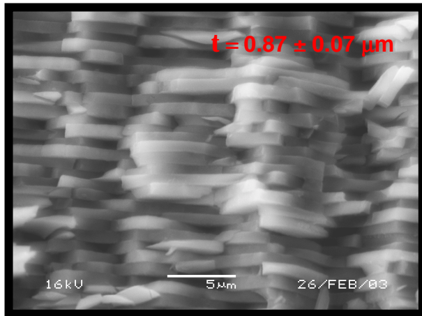
SEM : side view ceramic microlaminate columnar structure
