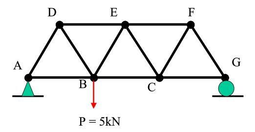
4. Calculate the forces in all members of the following truss, indicating whether each member is in tension or compression.
