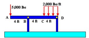
Hint: You will need to start off by drawing a Free Body Diagram for this problem, and determining the shear forces and bending moments.
