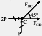
At point C, F<sub>BC</sub> can be split into its horizontal and vertical components, with  $[F_{BC}]_x = F_{BC} \cos 45^\circ$  and  $[F_{BC}]_y = F_{BC} \sin 45^\circ$ . That gives us only two vertical forces,  $[F_C]_v (=P)$  and  $[F_{BC}]_v$ . Thus,
