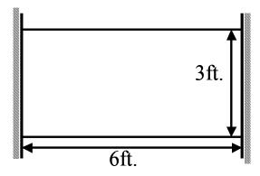
Since the cylinder is constrained by the walls in the x-direction (horizontal direction), we can say that the sum of all the strains in that direction must be zero, i.e.  $\varepsilon x = 0$ . We know that there will be a thermal strain,  $\varepsilon T$  due to the heating of the cylinder, and the cylinder
