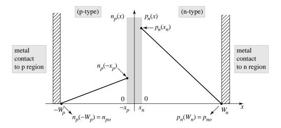
• Steady-state --> minority carriers must be continuously injected across the junction to keep  $p_n(x_n) >> p_{no}$  and  $n_p(-x_p) >> n_{po}$  while the same number is continuously extracted at the ohmic contacts
