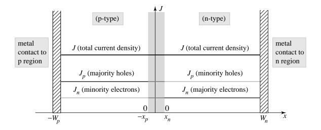
$$J = J_n + J_p = \left(\frac{qD_n n_{po}}{W_p - x_p} + \frac{qD_p p_{no}}{W_n - x_n}\right) \left(e^{V_D/V_{th}} - 1\right) = J_s \left(e^{V_D/V_{th}} - 1\right)$$
