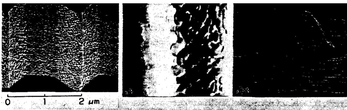
Figure 12.24: AFM images of grooves etched in Si for three increased magnifications. The highest magnification scans show the details of the groove substructure which is only  $50\text{\AA}$  high. (Y. Martin, C.C. Williams, and H.K. Wickramasinghe, *J. Appl. Phys.* **61**, 4723 (1987)).
