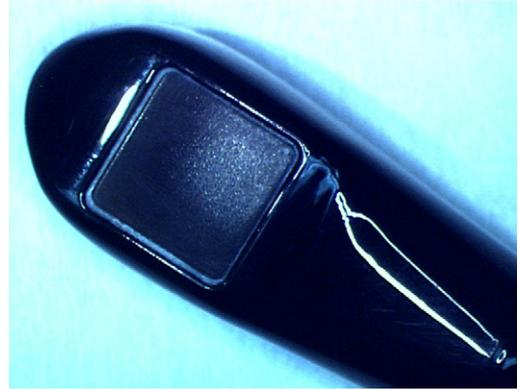
Fig. 2. A Matrix Array Transesophageal Transducer distal tip. The active aperture is 10 mm  $\times$  10 mm. Note that this supports 2D and 3D imaging, and spectral and color Doppler modes.
