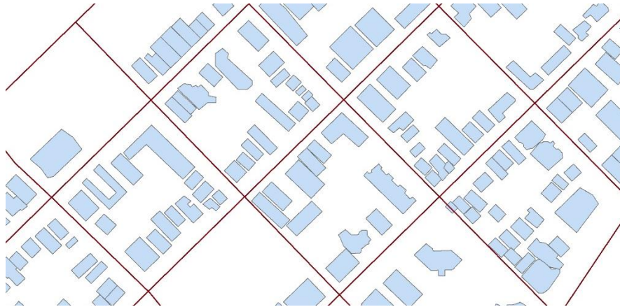
Fig.4.1. Objects required as input (polygons of buildings and street centerlines) in GIS.
