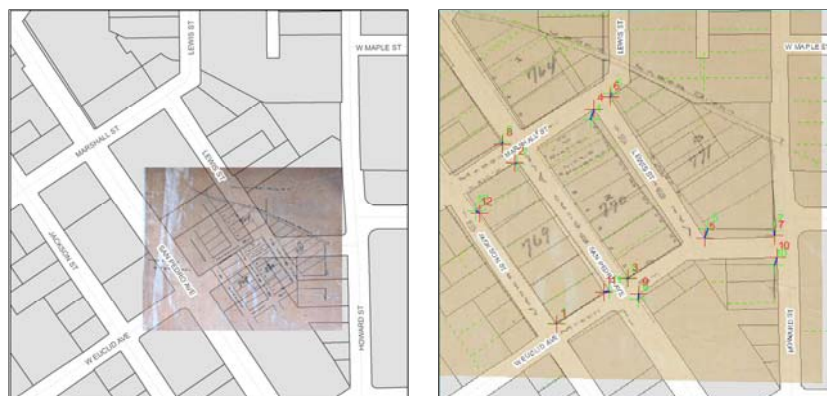
Fig. 2. (a) left & (b) right. A scanned map with the distortion, and after georeferencing/adjustment using control points.
