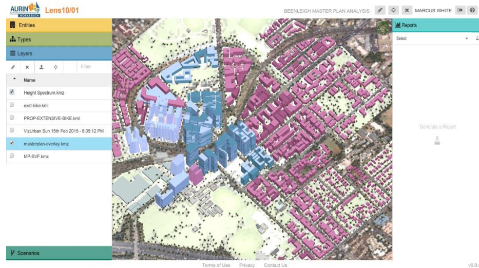
Figure 3 Overview of urban morphology indicating different precincts and zoning with indicative building volumes displayed in the Lens10, 3D urban design tool developed by MUTopia. Model built by White, Langenheimer, & Kimm using AURIN data and 2D GHD and Logan Council master plan data.
