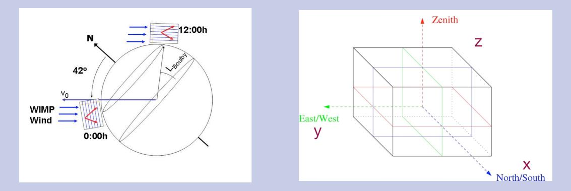
Anisotropy is maximised if normal to read-out plane is perpendicular to spin axis of Earth. This is the case for the x-z plane.
