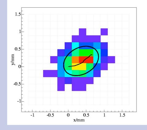
Below 20 keV tracks too short (<3-4 pixels) to reconstruct direction. (n.b. direction reconstruction threshold > recoil detection threshold and  $\neq$  background discrimination threshold).
