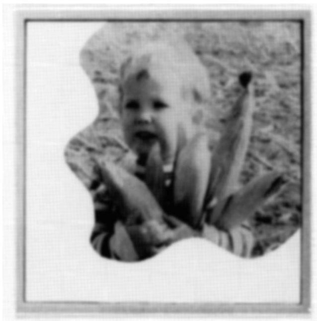
Figure 41 Photograph of a complex LPP/LCP retarder image on a single glass substrate visualized in transmission in white light between crossed polarizers. Only the part of the image confined between the crossed polarizers is visible, whereas the phase information outside remains invisible (white).
