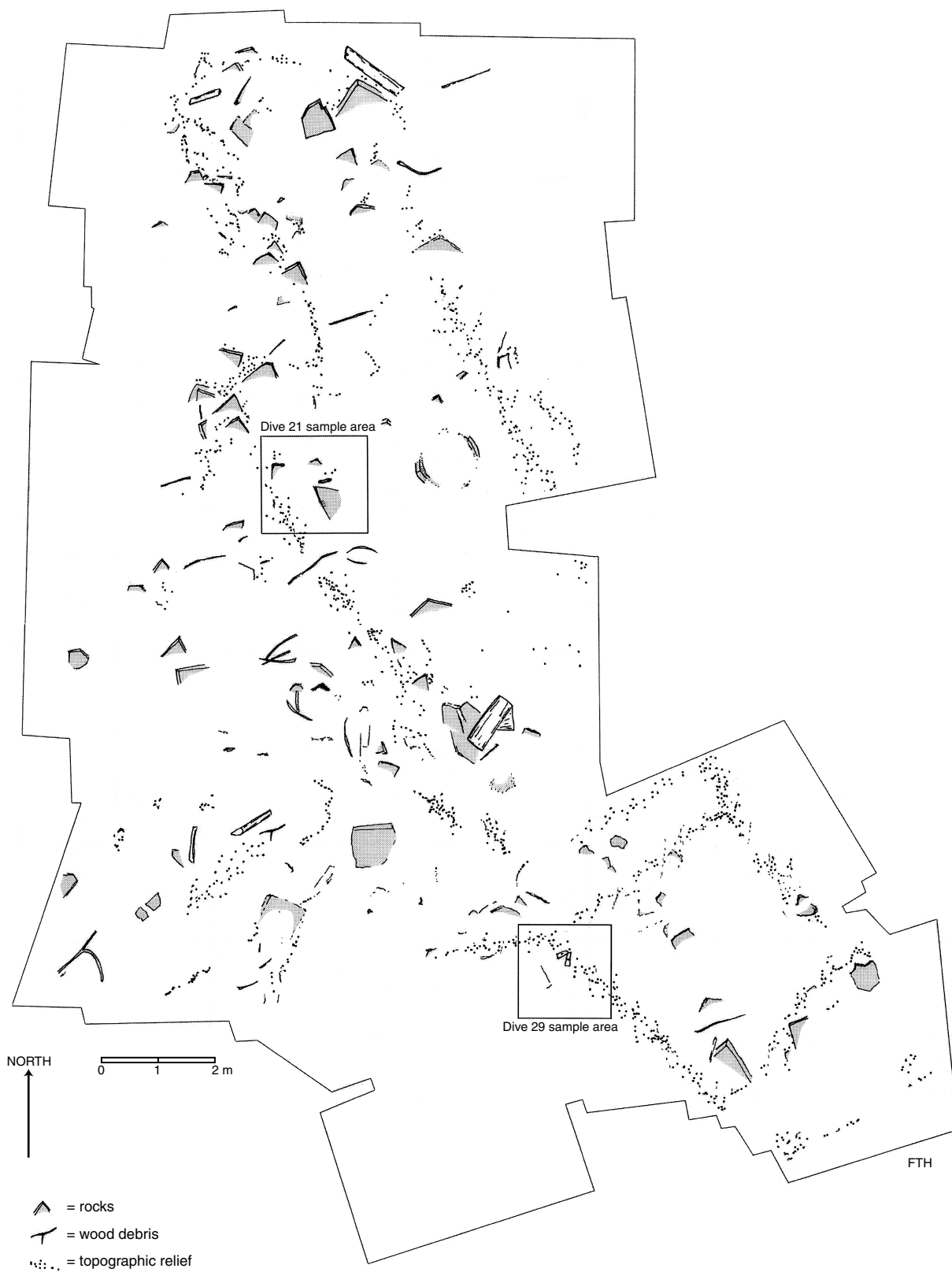
Fig. 13. Site 82 plan, based on a mosaic of 52 ESC images corrected for parallax distortion. Preliminary topographic relief based on stereoscopic pairing of ESC photos.
